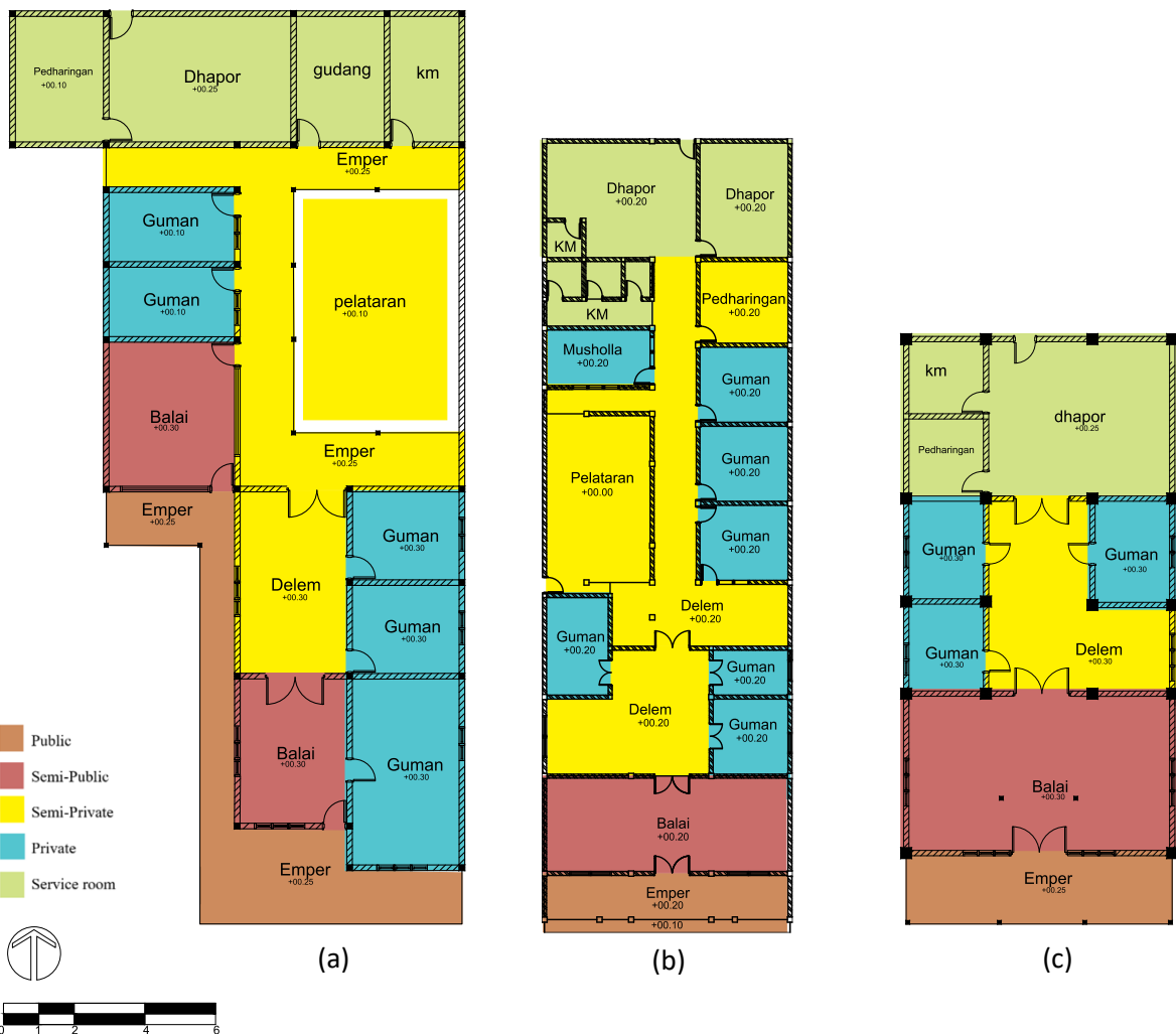
Figure 5. Labelling Proses in Pendalungan Community House. Art deco house (a), palemangan house (b), and Klening house (c)
